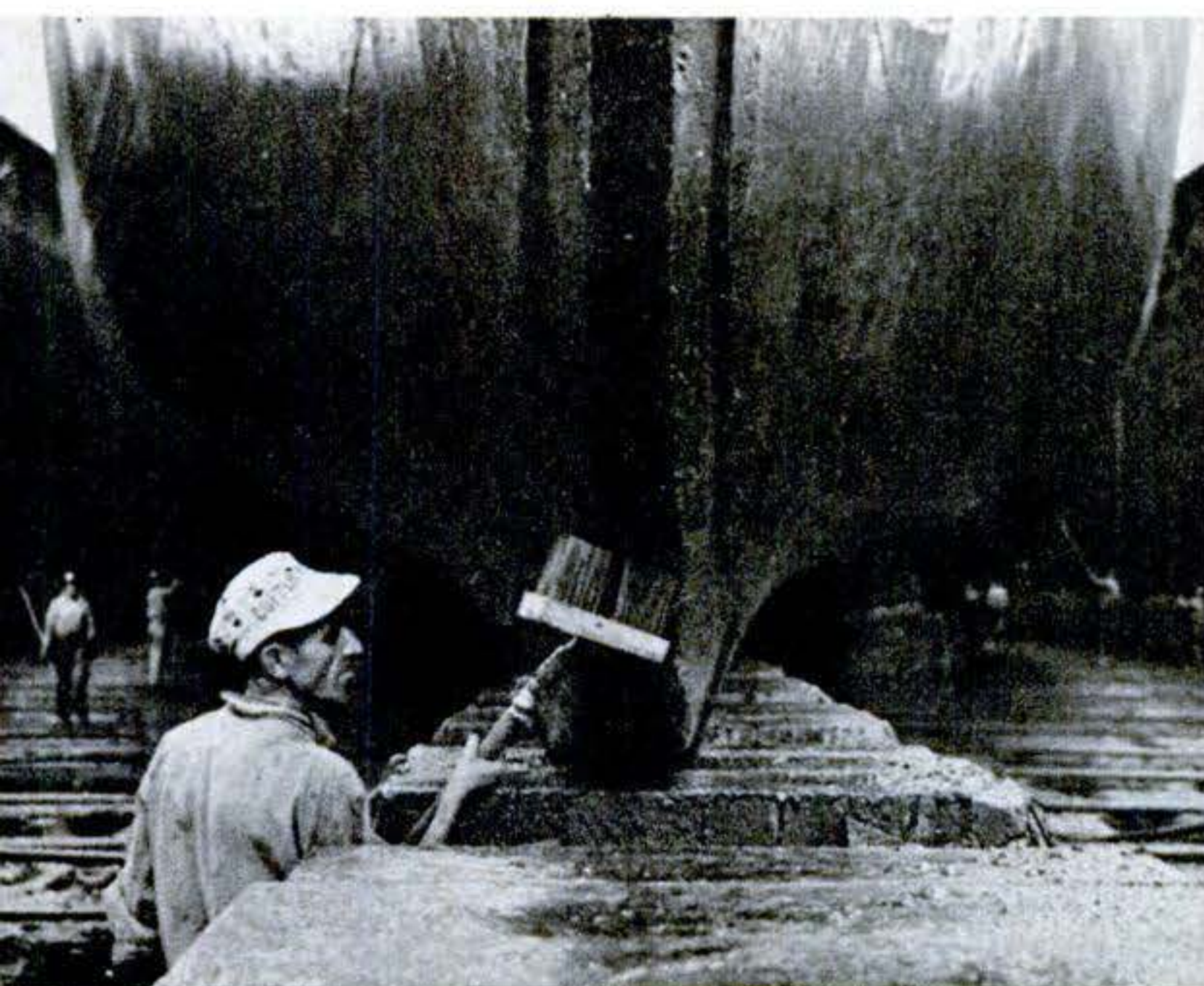
7. Barnacle's-eye view of bow of vessel gives unusual glimpse of underwater design of a big ship's keel as it rests on wooden blocks in dry dock. Note how successfully the ticklish job of centering the ship over the submerged keel blocks has been accomplished.
